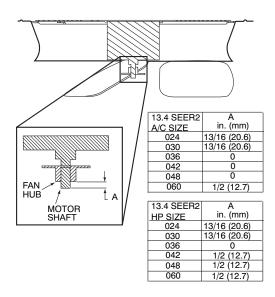
Fig. 19 - Outdoor Fan Adjustment
