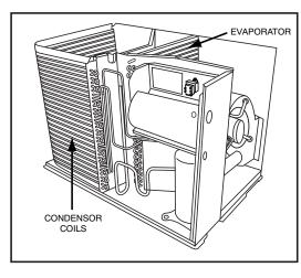
Fig. 8 - Access of Condenser Coil
