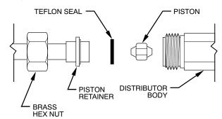
Fig. 24 – Refrigerant Flow-Control Device
