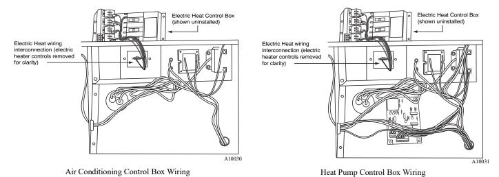
Fig. 31 – Control Box Wiring
