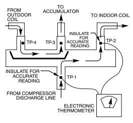
Fig. 21 – Reversing Valve (Heating Mode, Solenoid De-Energized)
