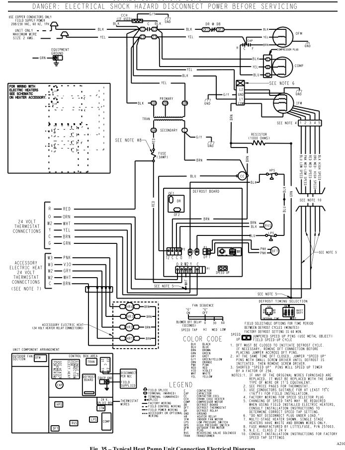
Fig. 35 - Typical Heat Pump Unit Connection Electrical Diagram
