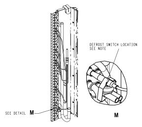
Defrost switch can either be located on the bottom of tube
