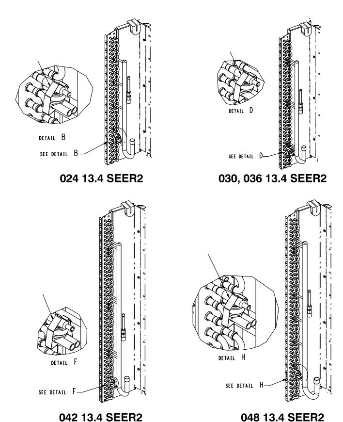
Defrost thermostat can either be located on the bottom of tube (as shown) or on the top and must not interfere with any other tubing.
