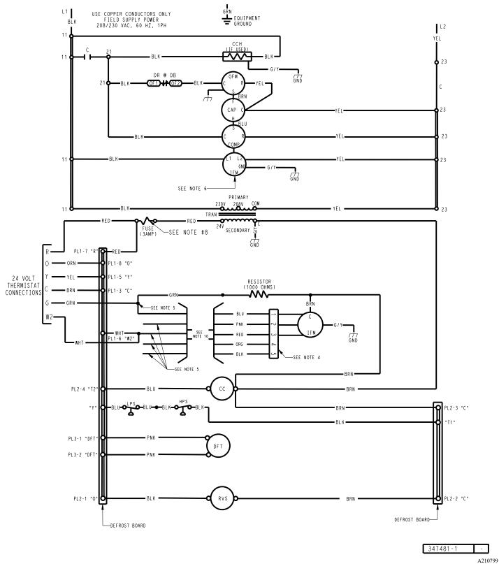
Fig. 36 – Typical Heat Pump Unit Ladder Electrical Diagram
