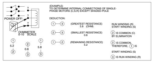
Fig. 18 – Identifying Compressor Terminals
