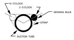
Fig. 23 - Position of Sensing Bulb
