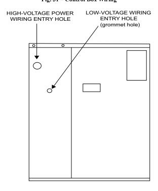
Fig. 32 – Unit Electrical Connection
