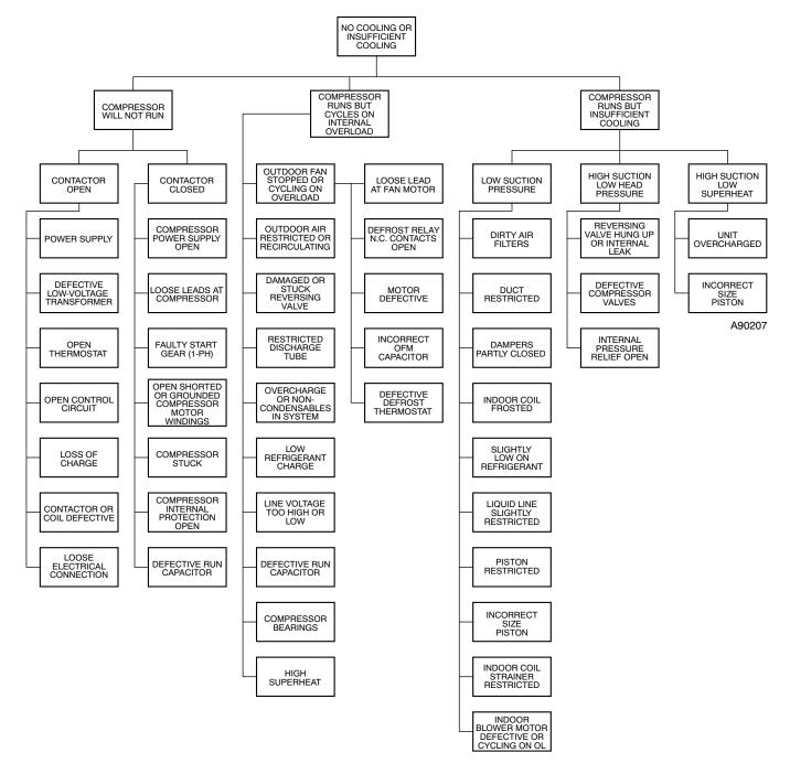
Fig. 39 – Heat Pump Troubleshooting - Cooling Cycle
