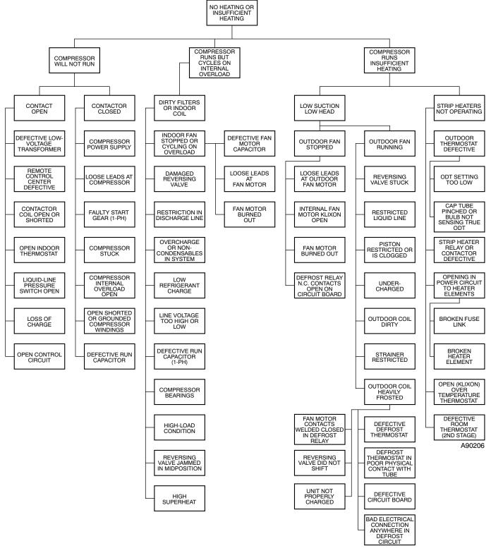
Fig. 38 – Heat Pump Troubleshooting - Heating Cycle
