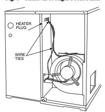
Fig. 7 - Removal of Right Side Back Panel
