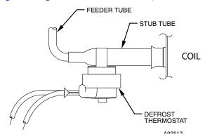
Fig. 13 – Defrost Thermostat Location
