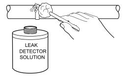
Fig. 26 – Bubble Leak Detection
