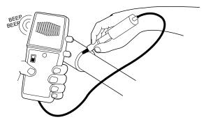
Fig. 25 - Electronic Leak Detection
