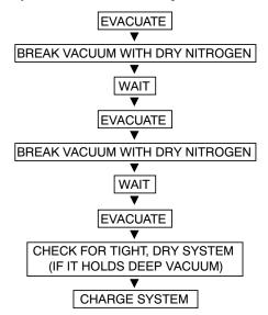
Fig. 28 - Triple Evacuation Method
